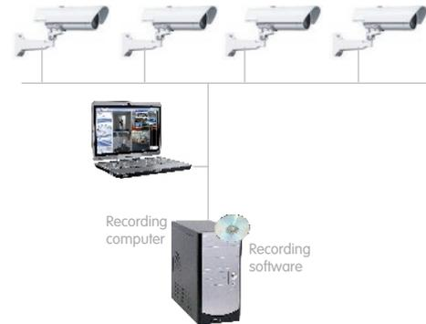
Combining high-resolution video with in-camera-recording means fewer cameras are needed and direct recording to any type of storage device such as, in-camera SD card, Hard Disk or NAS is possible.
