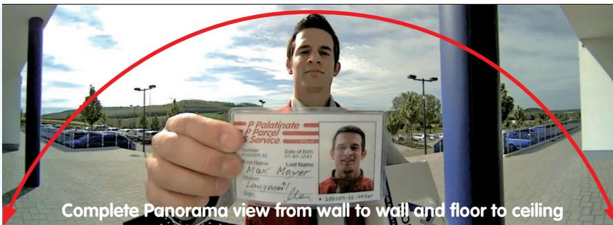
The MOBOTIX T24 captures a superwide 180° panorama view. 2-way audio/video communication and access control is possible from anywhere in the world! The T24 is based on the international video telephony standards VoIP/SIP and H.264 – the latest telephony standard after ISDN and analog.
