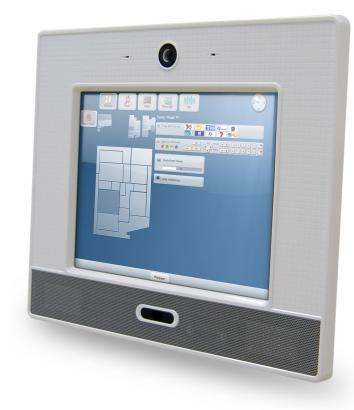
15" Embedded Interface connects to an Embedded Server via a single network cable providing an all-in-one additional interface option.
