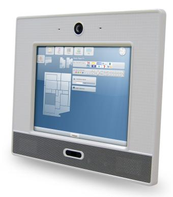
The Embedded Server is the centre of the Automation network - housing all the data including macros, logic and interface information in one slimline recessed wall mount unit.
