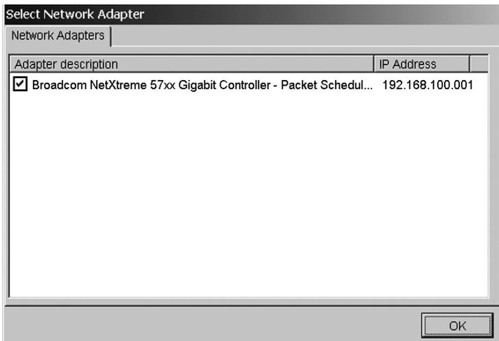
Figure 18. Select the network adapter used to connect to the C-Touch Colour
