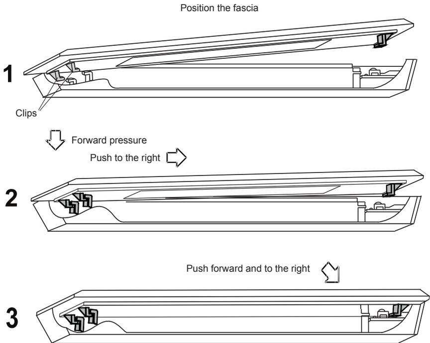
Figure 12. Attaching the fascia.
