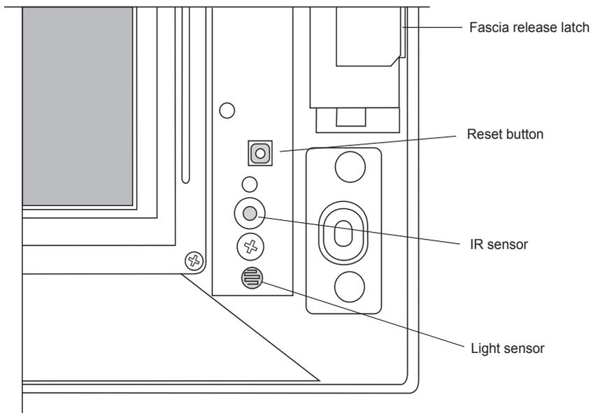
Figure 27. The reset button is located underneath the fascia
