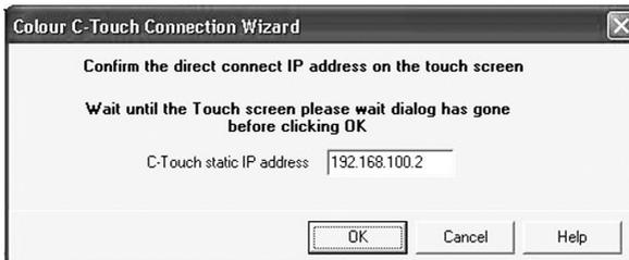
Figure 20. An IP Address will be suggested for the touch screen
