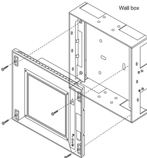
Figure 11. 4 screws hold the touch screen in place.
