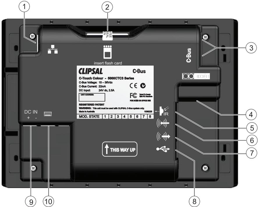
Figure 2. Back panel connection points.
