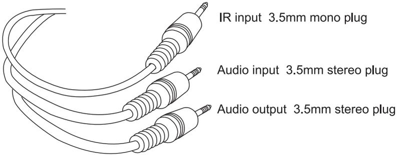
Figure 14. Audio and IR cable plugs
