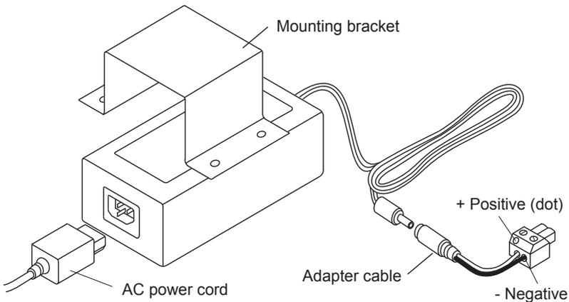
Figure 15. Power supply and adapter.
