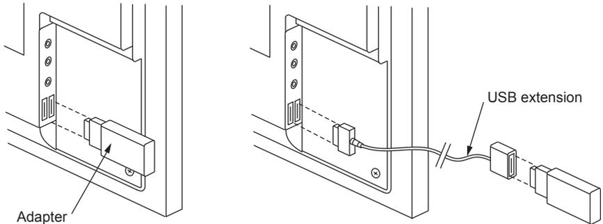
Figure 16. USB device and extension cable.
