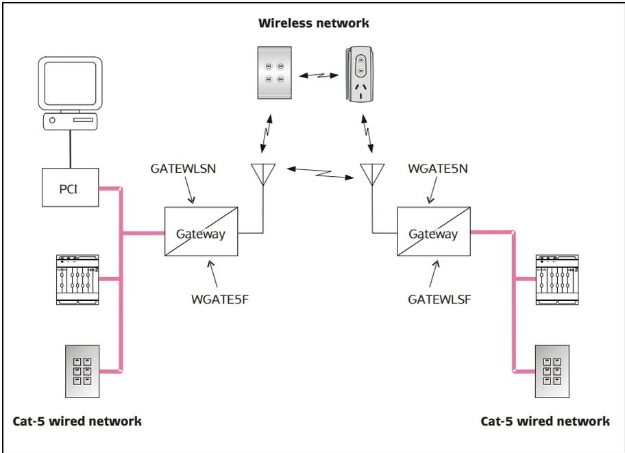
Figure 4 – Identification of Gateways when scanning from a PCI
