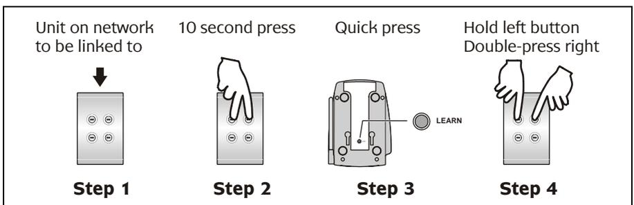
Figure 2 – Connecting the Gateway to a wireless network
