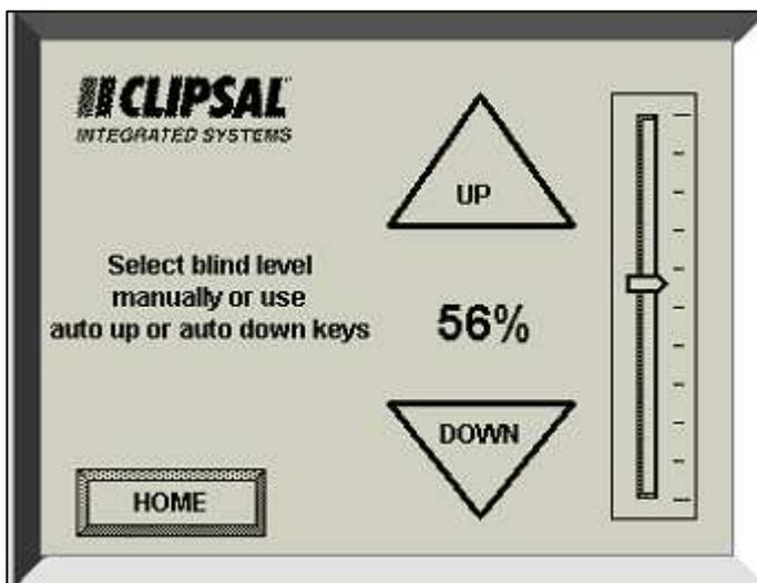
The slider is programmed as a “slider key function” controlling the group of the blind assigned to the shutter relay.
