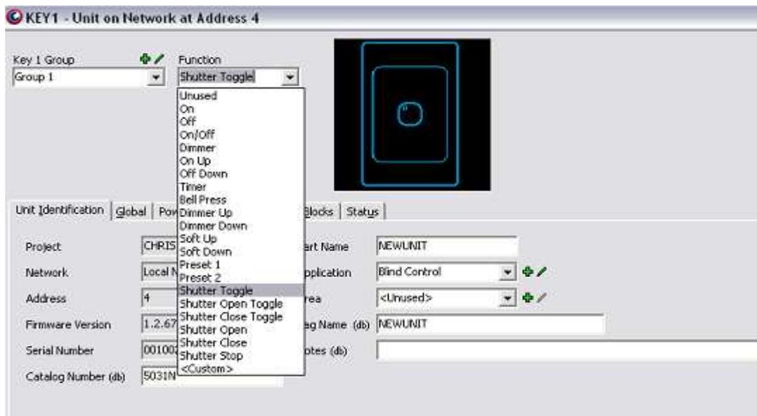
When using a touch screen the Shutter Macro Functions may be emulated using the Preset and the Ramp Off key functions, select the Ramp Rate to be slightly less than the failsafe time for correct operation of the ramp off key. Select the group address and the shutter relay and enter the preset levels as below;
