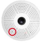
The LED now flashes once and repeats the flash signal after pausing for one second (the number of flashes indicates the current boot option). To go to the next boot option, briefly press the key again (< 1 sec). After the last boot option, the camera returns to the first option (LED flashes once).
