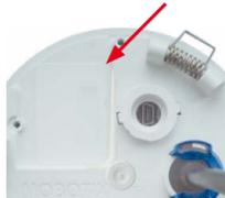
Carefully push the module board onto the receptacle.
