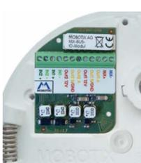
When attaching the connection wires to the MxIOBoard-IC, make sure the wires are guided to a cable tie and tie the wires to the network cable, for example).
