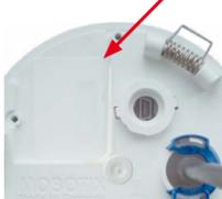
Carefully push the module board onto the receptacle.
