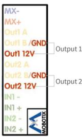
To use one or both signal outputs not as potential-free outputs (for relays), but as **12 V outputs**, open the **Admin Menu > Hardware Configuration > Manage Hardware Expansions** dialog. In the **MxBus/IO Board** section, click on **Connect** for each output you want to use.
