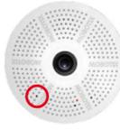
The LED now flashes once and repeats the flash signal after pausing for one second (the number of flashes indicates the current boot option). To go to the next boot option, briefly press the key again (< 1 sec). After the last boot option, the camera returns to the first option (LED flashes once).
