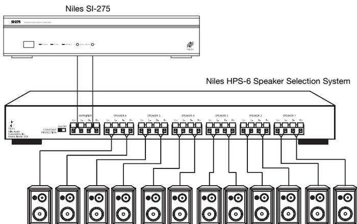
Speaker selection systems allow each pair of speakers to be turned on and off from your equipment location (or even via remote control).
