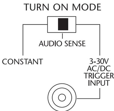
**Constant** - The auto turn-on circuitry is off. The front panel master power switch operates the amplifier. In is "On", out is "Off".
