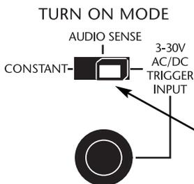
Slide the switch with your fingernail or a 1/8" slotted screwdriver blade.
