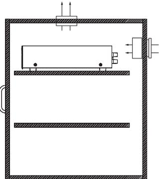
If the cabinet rear is not open to fresh air or if you're using low impedance loads, install two "boxer fans" (55cfm fan) to provide continuous air flow into and out of the cabinet.
