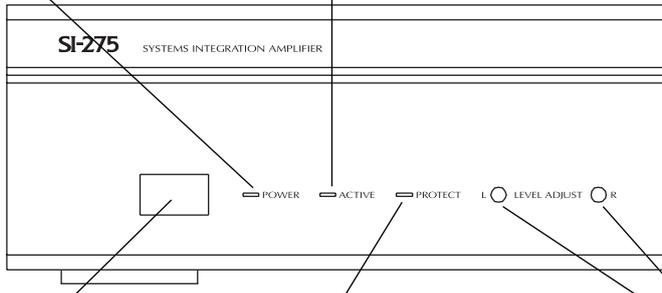
Front panel "Master Power" switch turns off the entire amplifier, including the Turn-On circuitry.
