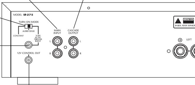
3.5mm Mini Plug socket for 12v DC Control output.
