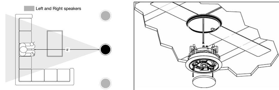
Figure 1. Typical placement for a surround system
