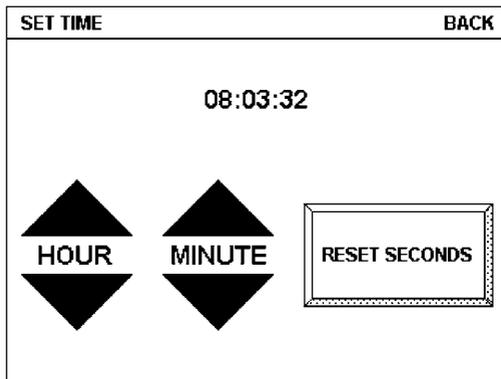
If your C-Touch unit is not displaying the correct time you can use this page and adjust the hour and the minute with the triangular buttons. By pressing the upward pointing triangle in the hour section, you can increase the hour displayed. The touchscreen uses a 24-hour clock for setting the time.
