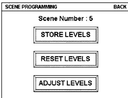
The “Reset Levels” button resets the current scene as originally designed. Pressing the “Store Levels” button will store the current levels (which may be set by any means, such as walking around and setting levels by eye). The “Adjust Levels” button allows manual adjustment of the levels in the scene. Pressing this button will produce this screen:
