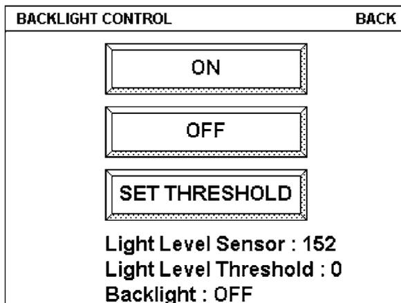
The remaining two buttons labelled "ON" and "OFF" allow you to temporarily turn the backlight on or off. The last line on the screen, labelled "Backlight:" indicates the actual state of the screen.
