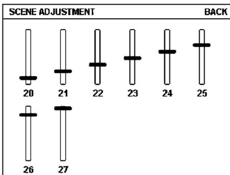
Each load in the scene is accorded a slider with a label showing its group address in Hexadecimal. If more loads are included in the scene than can be accommodated on the screen then the upper right hand corner will show a “next” button to see the rest of the loads.
