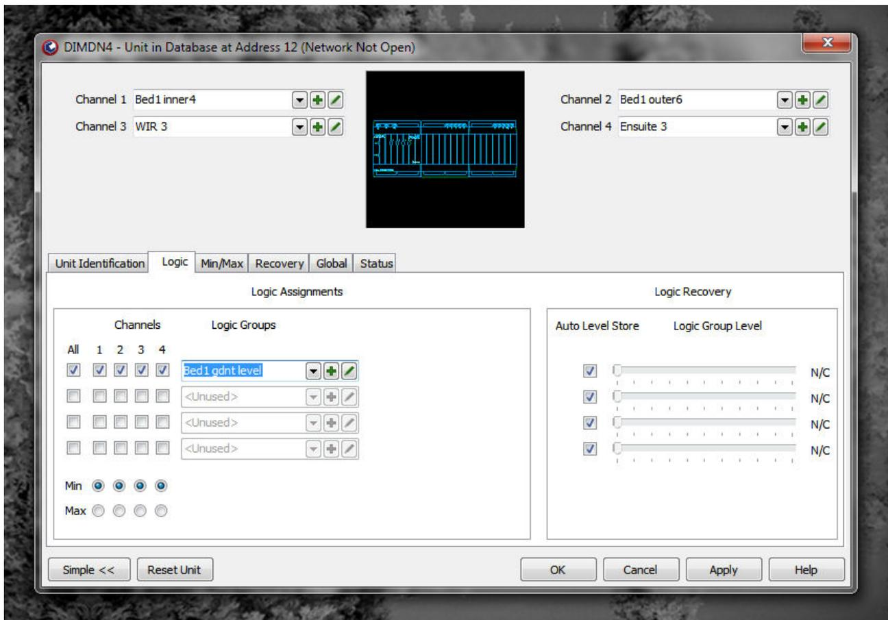
**Figure 2.** C-Bus Toolkit software GUI for programming a 4 Ch dimmer, showing the Logic tab.
