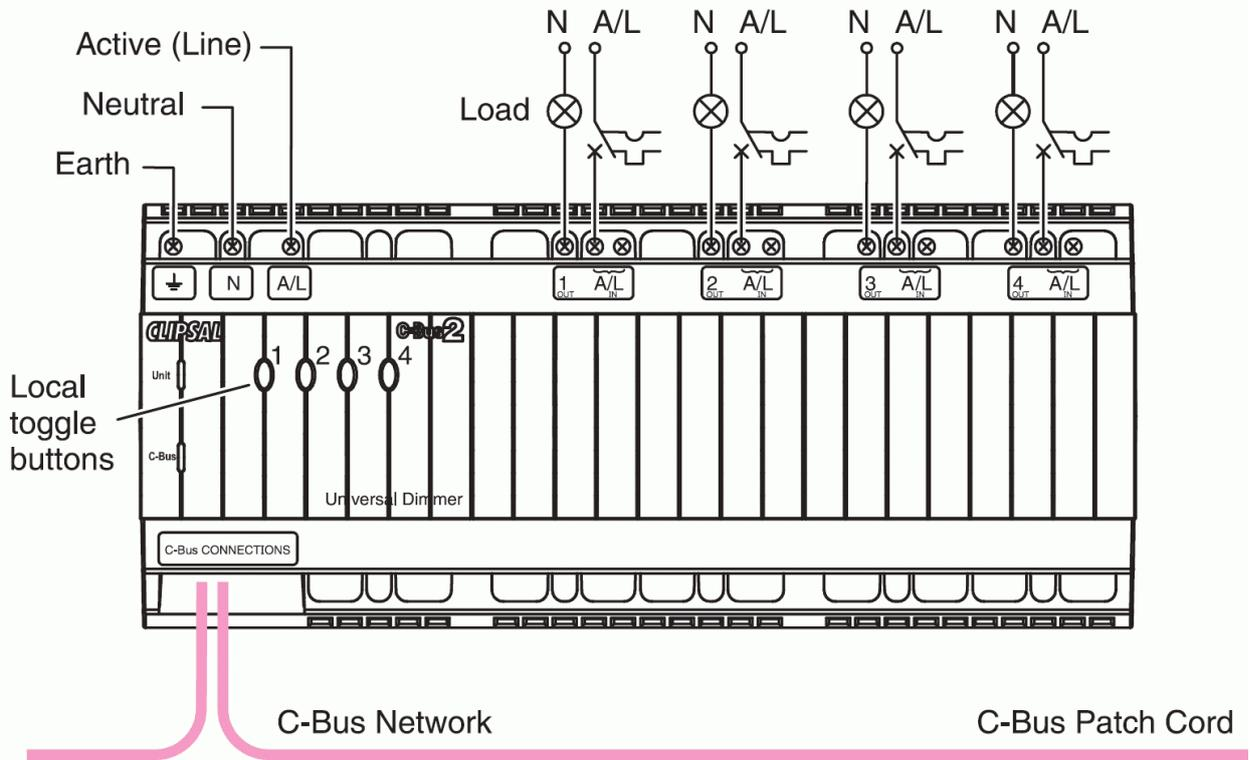
**Figure 1.** C-Bus L5504D2U 4 Channel C-Bus dimmer, with a dimmer output for each Channel.
