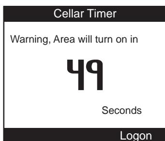
The system also allows a warning timer to be programmed for each Area that has a deferred arming timer.
