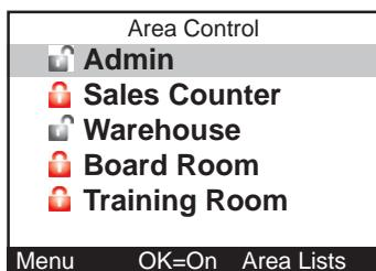
The Area Control screen is now displayed, with the first Area (or Area List) that you are allowed to control highlighted, and a text prompt for the relevant action on that Area, shown at the bottom of the screen. i.e. “OK=On”
