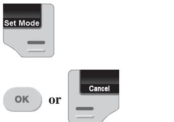
The <Set Mode> FUNCTION key can be used to choose the timer mode. Options will vary depending on the type of entity being controlled.
