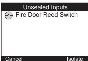
After pressing the <ON> key, the display may show a message like this. It means that any items displayed are either in an alarm state or faulty, and the Area will not turn ON.
