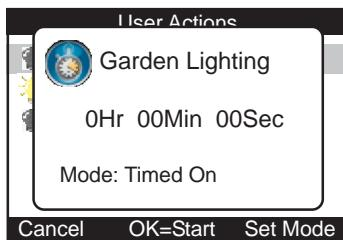
If “Timed” is selected, use the <LEFT> and/or <RIGHT> ARROW keys to position the cursor on the time digit you wish to edit, then use the SCROLL WHEEL or the ALPHA-NUMERIC keys to enter the required value.
