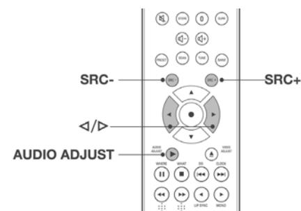
The adjustment range for bass and treble is -7 to +7, with neutral being 0.
