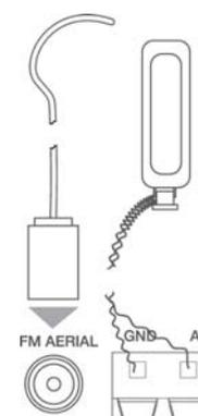
You may have to experiment with the position of the AM aerial to obtain the best reception. The end of the FM aerial should be connected to a wall as high as the length of the aerial will allow. As with the AM aerial, you may have to experiment with its positioning to obtain the best reception.
