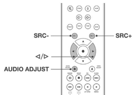
This function allows you to shift the balance between the left and right loudspeakers.
